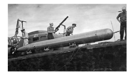
A modern torpedo is an underwater ranged weapon launched above or below the water surface, self-propelled towards a target, and with an explosive warhead designed to detonate either on contact with or in proximity to the target. Historically, such a device was called an automotive, automobile, locomotive, or fish torpedo; colloquially a fish. The term torpedo originally applied to a variety of dev... Wikipedia
